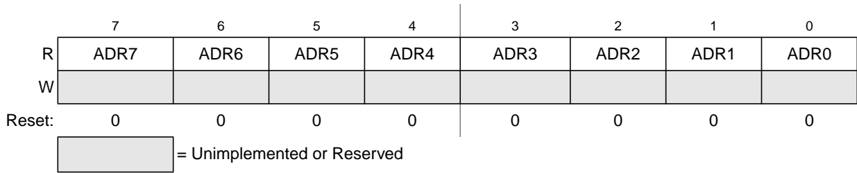
Figure 9-7. Data Result Low Register (ADCRL)
